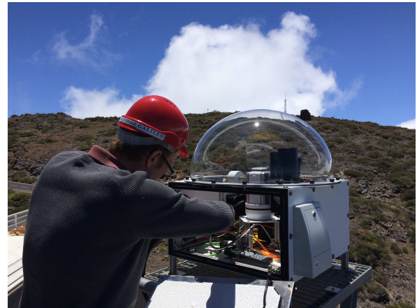
Figure 3. Left: Solar telescope schematic: a 200 mm focal length, 3 inch aperture lens focuses light into an integrating sphere whose output is fiber-coupled to the calibration unit of the HARPS-N spectrograph. The telescope tracks the Sun using an amateur alt-az mount. Guide cameras built from commercial CMOS cameras provide images of the Sun and provide feedback to keep the telescope centered on the solar image. Right: Alex Glenday completes installation of the solar telescope at the TNG.
